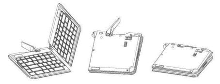
4. Push the handle on the top of the keyboard, back into the closed and locked position.
