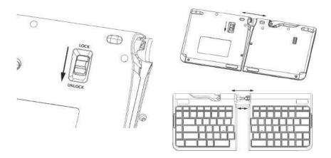
2. Once the two keyboard halves have been separated, release the handle on the top of the keyboard.
