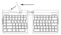
3. Next, you're going to push the two keyboard segments into the closed and locked position. To do this, push and hold the Lock button on the back of the keyboard to the Unlocked position, now push the two segments of the keyboard together until you can no longer see the folding hinge.
