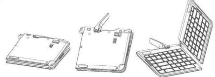
2. When the keyboard is unfolded, push the handle lever on the top of your keyboard back into the closed and locked position.
